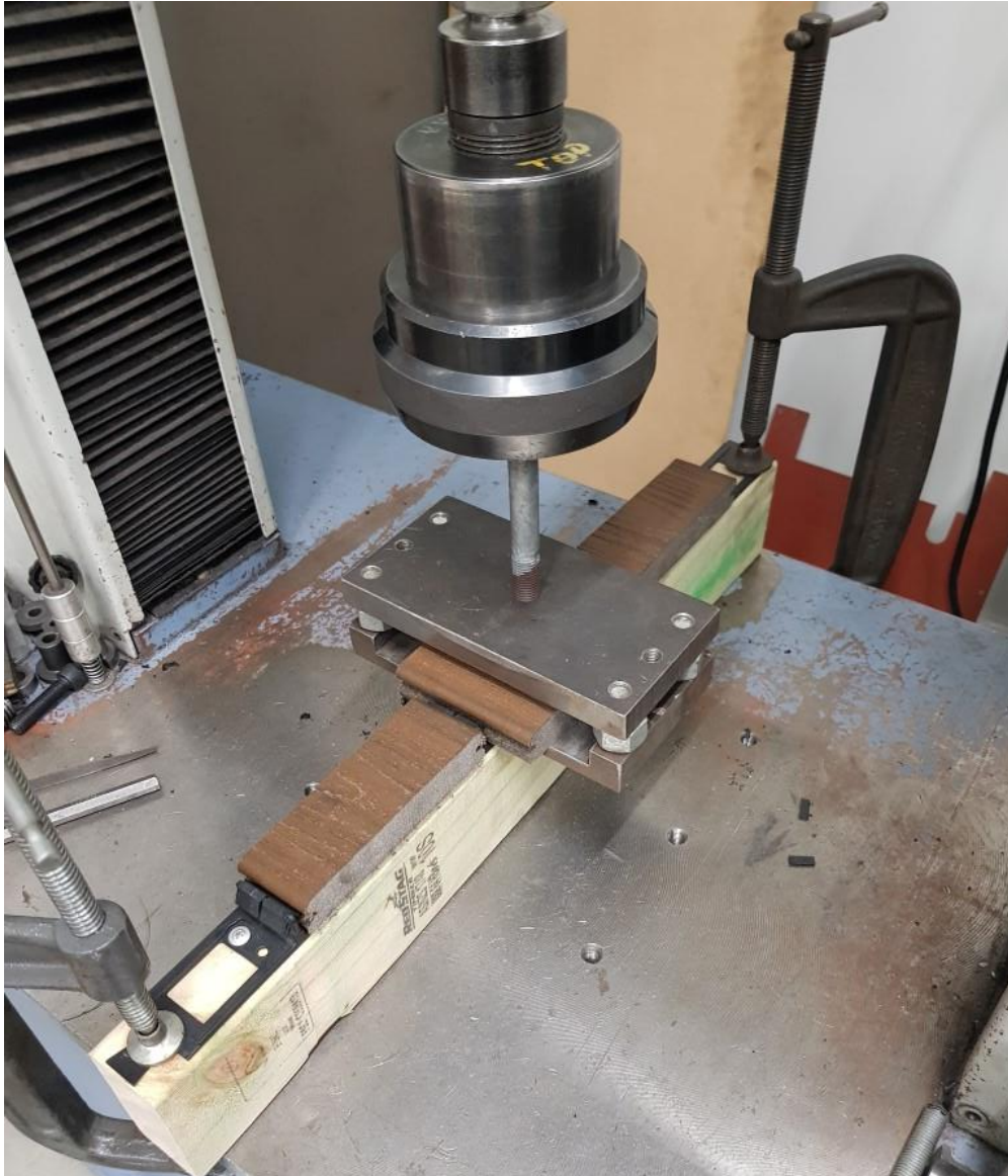
Figure 2: Test setup used to test middle plank configuration.
