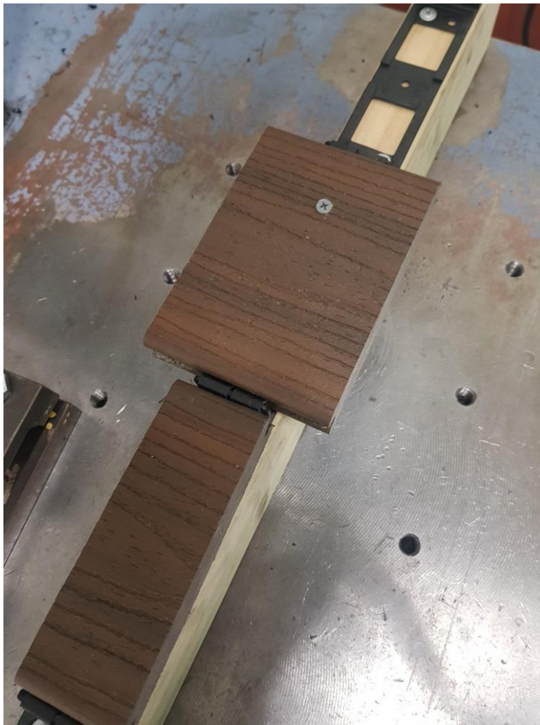
Figure 1: Installation method used for cyclone edge configuration.
