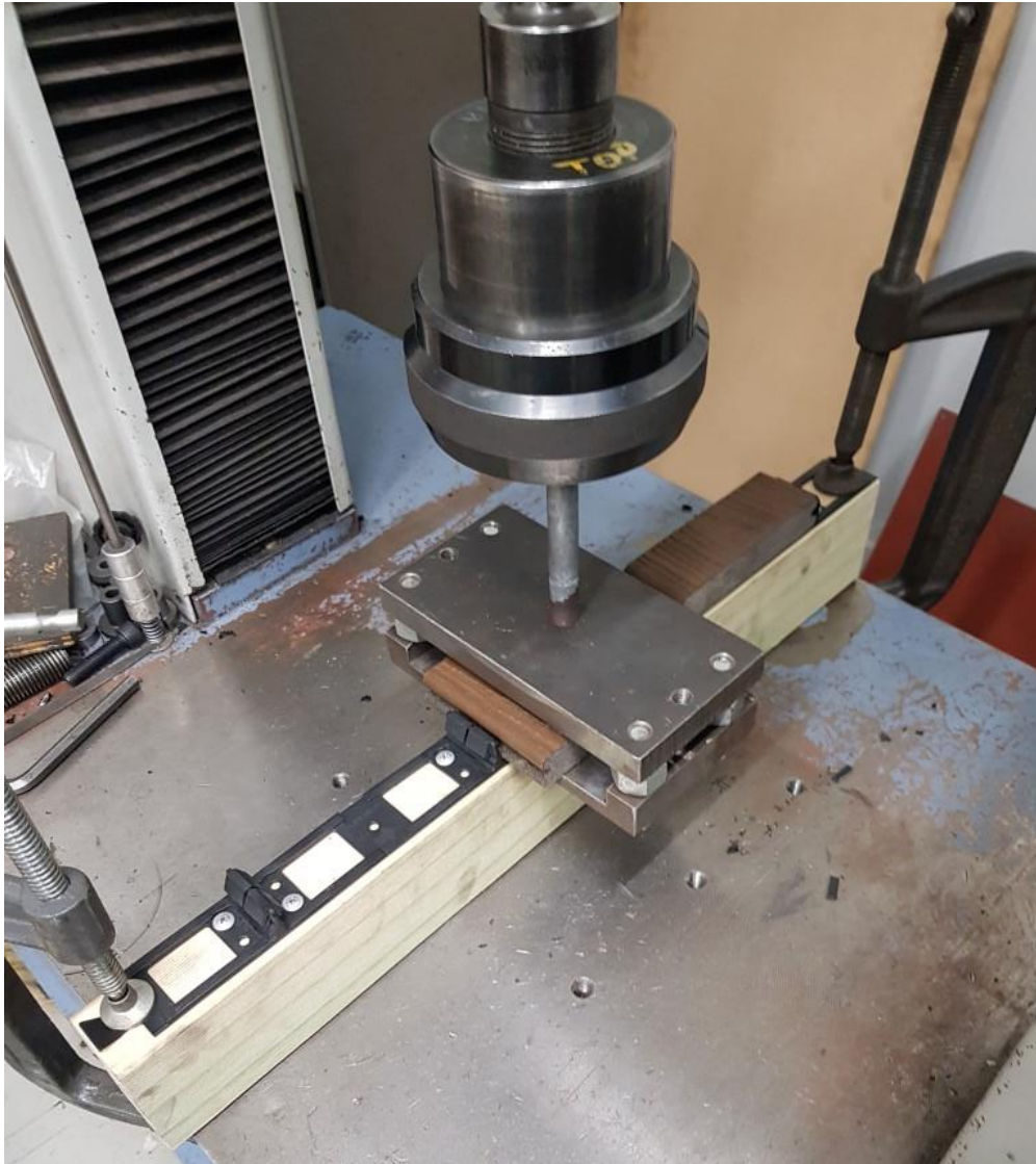
Figure 3: Test setup used to test edge plank configuration.
